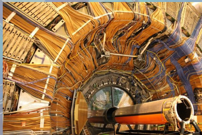
Forward detector designed for B-physics
